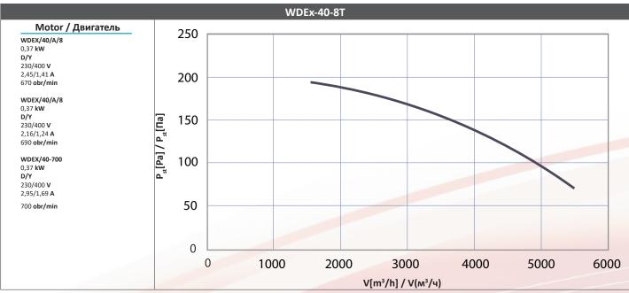
Pst –static pressure in the fan inlet
