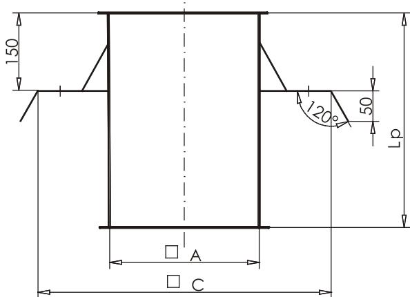
Roof bases are made of galvanized steel sheets.
