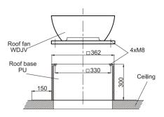
Universal roof base PU and damping roof base PUT for all fan sizes
